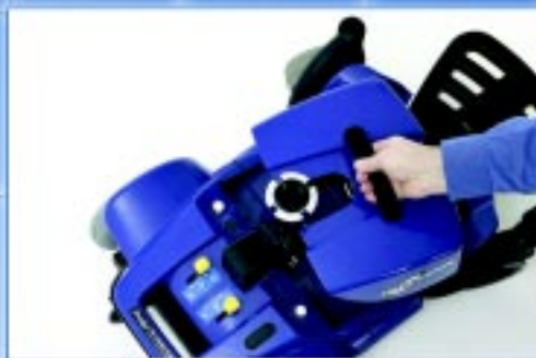
Easy to remove battery pack
